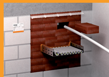
Simple retroinstallation through removal of individual blocks.
