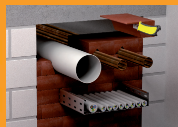
Running of combustible pipes without additional measures.
