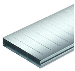
Underfloor duct (2 piece) for routing cables in screed-covered underfloor systems, according to EN 50085-2-2. Removable and continuously lockable trunking lid. With separating retainer in the trunking base. Only compatible with the UZD250-4/350-4.
