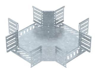
Cross-over for the creation of a horizontal branch, fitting for lock and screw-on cable trays of side height 110 mm. Screwless mounting with double clamps or screw connection with FRS truss-head screws and M6 combination nuts. Can be used indoors and outdoors. Fastening material must be ordered separately.
