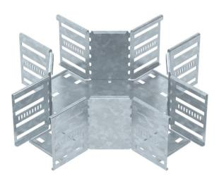
Cross-over for the creation of a horizontal branch, fitting for lock and screw-on cable trays of side height 110 mm. Screwless mounting with double clamps or screw connection with FRS truss-head screws and M6 combination nuts. Can be used indoors and outdoors. Fastening material must be ordered separately.
