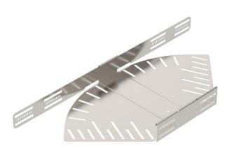
Angle-adjustable bend for the creation of a horizontal branch, fitting for lock and screw-on cable trays of side height 60 mm. Adjustable angle 0–90°. Screwless mounting with double clamps or screw connection with FRS truss-head screws and M6 combination nuts. Can be used indoors and outdoors. Fastening material must be ordered separately.
