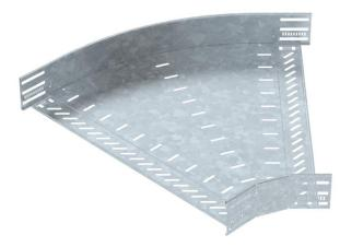
45° bend for the creation of a horizontal branch, fitting for lock and screw-on cable trays of side height 85 mm. Screwless mounting with double clamps or screw connection with FRS truss-head screws and M6 combination nuts. Can be used indoors and outdoors. Fastening material must be ordered separately.
