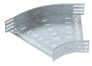
45° bend for the creation of a horizontal branch, fitting for lock and screw-on cable trays of side height 85 mm. Screwless mounting with double clamps or screw connection with FRS truss-head screws and M6 combination nuts. Can be used indoors and outdoors. Fastening material must be ordered separately.
