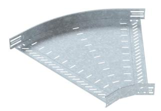
45° bend for the creation of a horizontal branch, fitting for lock and screw-on cable trays of side height 60 mm. Screwless mounting with double clamps or screw connection with FRS truss-head screws and M6 combination nuts. Can be used indoors and outdoors. Fastening material must be ordered separately.
