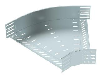
45° bend for the creation of a horizontal branch, fitting for lock and screw-on cable trays of side height 110 mm. Screwless mounting with double clamps or screw connection with FRS truss-head screws and M6 combination nuts. Can be used in indoor areas. Fastening material must be ordered separately.
