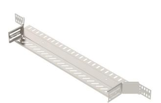
Add-on tee for the creation of a horizontal branch or cross-over, fitting for lock and screw-on cable trays of side height 60 mm. Screwless mounting with double clamps or screw connection with FRS truss-head screws and M6 combination nuts. Can be used indoors and outdoors. Fastening material must be ordered separately.
