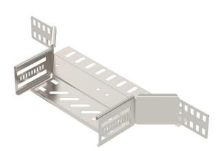
Add-on tee for the creation of a horizontal branch or cross-over, fitting for lock and screw-on cable trays of side height 60 mm. Screwless mounting with double clamps or screw connection with FRS truss-head screws and M6 combination nuts. Can be used indoors and outdoors. Fastening material must be ordered separately.
