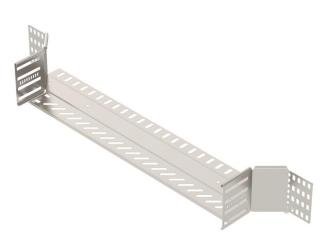
Add-on tee for the creation of a horizontal branch or cross-over, fitting for lock and screw-on cable trays of side height 110 mm. Screwless mounting with double clamps or screw connection with FRS truss-head screws and M6 combination nuts. Can be used indoors and outdoors. Fastening material must be ordered separately.
