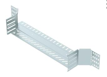
Add-on tee for the creation of a horizontal branch or cross-over, fitting for lock and screw-on cable trays of side height 110 mm. Screwless mounting with double clamps or screw connection with FRS truss-head screws and M6 combination nuts. Can be used in indoor areas. Fastening material must be ordered separately.
