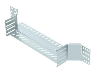
Add-on tee for the creation of a horizontal branch or cross-over, fitting for lock and screw-on cable trays of side height 110 mm. Screwless mounting with double clamps or screw connection with FRS truss-head screws and M6 combination nuts. Can be used in indoor areas. Fastening material must be ordered separately.
