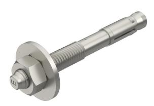
Bolt tie BZ for the anchoring of medium-duty to heavy-duty loads, indoors and outdoors, both in cracked and non-cracked concrete. It combines high approved loads with small edge distances and axial spacings.
