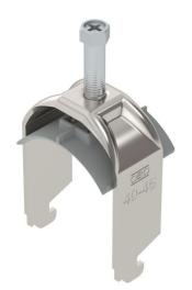
Clamp clip with N-foot, plastic pressure sleeve made of polypropylene. For vertical and horizontal mounting of 1 single cable on a C-profile rail. For slot width 11–12 mm With 1-start screw thread on pressure sleeve, universal hexagonal screw head WAF10, with slot and cross recess. Suitable for assembly indoors and outdoors. We recommend the use of a counter-sleeve.
